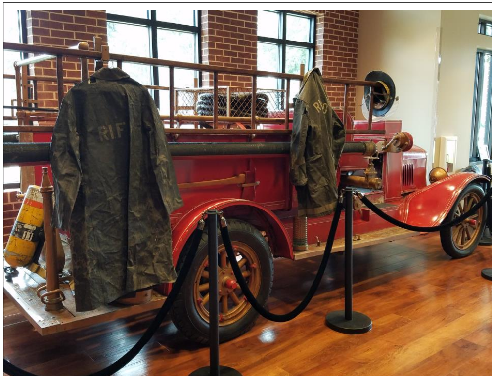
In 1925 Richmond purchased its first piece of motorized equipment, a Model "T" Ford fire truck known as "Old Tin sides" and was given the name No.1. It was equipped with all standard equipment, including a 50 gallon booster tank.
