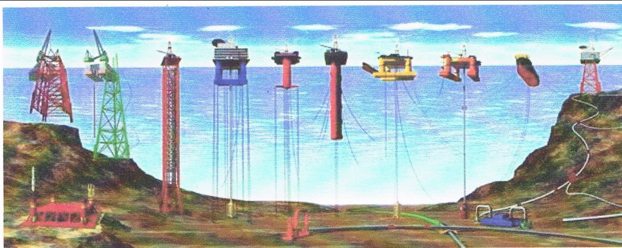
Modern offshore structures include (from left to right): 1 and 2 are conventional fixed platforms; 3 is a compliant tower; 4 and 5 are vertically moored tension leg and mini-tension leg platforms; 6 is a spar platform; 7 and 8 are semi-submersibles; 9 is a floating production and offloading facility; 10) sub-sea completion and tie-back to host facility.
