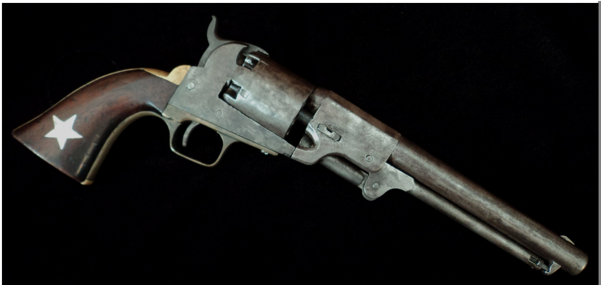
Distinctive Dance Brothers .44 caliber civil war revolver manufactured without a recoil shield giving it a flatter appearance.
